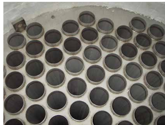
Photo-19 Top of heat exchanger (heat-release side gas is introduced into the tubes)
