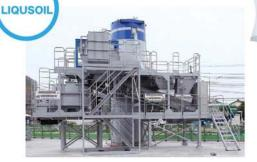
Surplus Soil Fluidized Treatment Facility for Subsurface Backfilling
