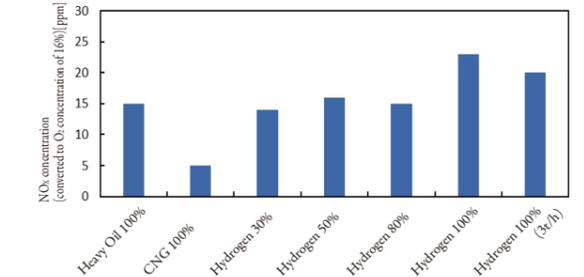
Figure 2: Results of NO<sub>x</sub> concentration (converted to O<sub>2</sub> concentration of 16%)
