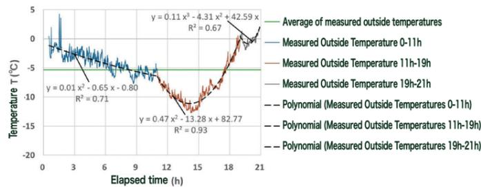
FIG. 7: Measured Outside Temperatures and Approximation Function
