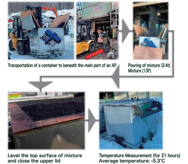
FIG. 3: Test Procedure
