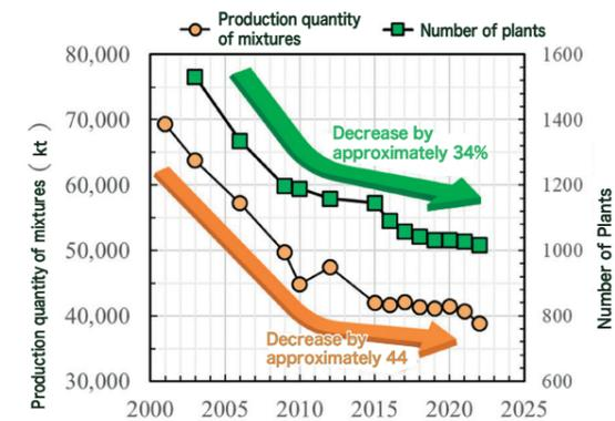
FIG. 1: Changes in Production Quantity of Mixtures and Number of Plants (Cited and edited from "2022 Asphalt Mixture Statistics Annual Report<sup>4)</sup>")
