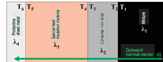
FIG. 8: Container Structure (Schematic diagram)
