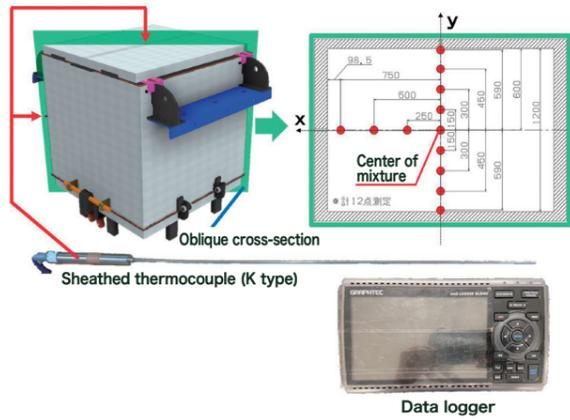
FIG. 4: Details of Measurement Points and Devices Used
