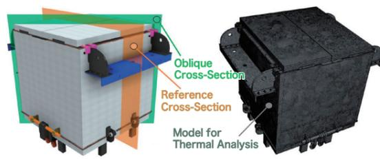
FIG. 6: 3D model and Defined Cross-Sections
