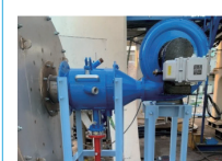
Started development of the world's first asphalt plant equipped with a hydrogen burner using hydrogen converted from ammonia (2022)
